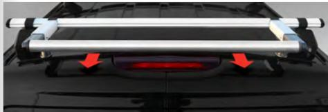
The KammBar<sup>™</sup> rear roller retains the same virtues as the KammBar<sup>™</sup> of both strength and modern styling combined, with features such as adjustable supports to allow for the optimum position of the stainless steel roller.
